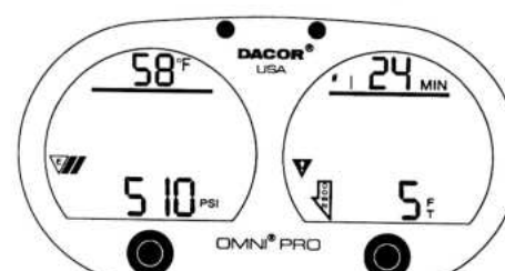
Fig. 19- If the 10 foot decompression stop is not reached within 2 minutes and 30 seconds, the Omni Pro will enter the Gauge Mode as illustrated and prevent diving for 24 hours after the dive is complete.
