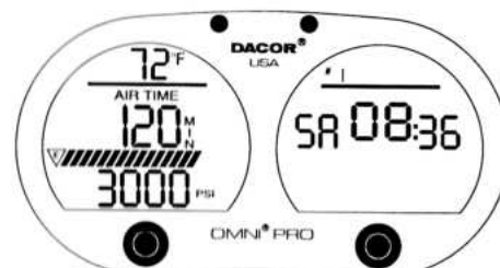
Fig. 22- The "SA" (saturation) display calculates the number of hours until residual nitrogen is off gassed. NOTE: For flying after diving, if the "SA" display is greater than the "FL" display, wait until the "SA" display clears to further reduce the risk of decompression sickness. The pressure side shows a new tank has been turned on.
