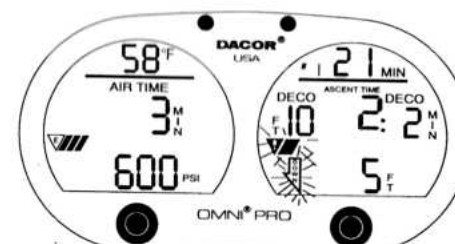
Fig. 18- Warning! The decompression stop has been omitted and the flashing "DOWN" arrow has appeared directing the diver to descend back to 10 feet for 2 minutes.
