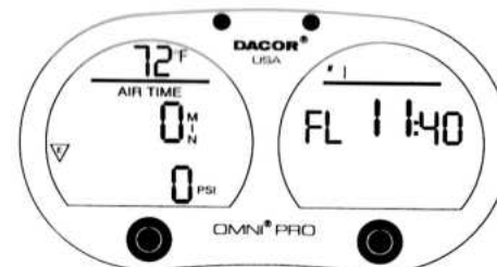
Fig. 21- "FL" counts down the minimum 12 hour wait before flying. The display shows 11 hours and 40 minutes remain after the elapsed surface interval time of 1:20. The tank has been removed and air time and PSI are both 0.
