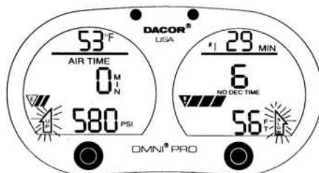
Fig. 13- The "SLOW" arrow will appear, on the right side, if the ascent rate is exceeded. This display shows a fast ascent was made when air time reached "0".
